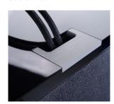
Pluggable cable inlet, made from aluminum EN AW-5083 in natural E6/CO anodized finish, with an integrated brush on top of the audio furniture.
